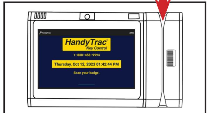
Use the biometric fingerprint reader **OR** scan your badge and type in your PIN. You must be signed in to the system to pull or return any key. Fingerprint access is only available on the HandyTrac Touch Premium.
